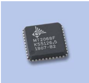
MT2068 Single-Chip Broadband Tuner
